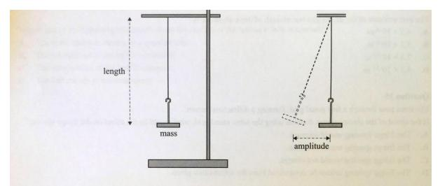
The students use a constant mass and a constant amplitude of swing, changing only the length of the pendulum and then measuring the time for five oscillations. They obtain four different time readings for four different lengths of the pendulum.
