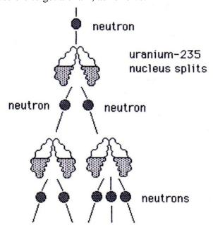
As this reaction continues more and more neutrons are produced increasing the chance of fission occurring. And of course an enormous amount of energy is released. However if the mass of the Uranium is too small most of the neutrons will escape. For an uncontrolled reaction to occur, the material available for fission must be above a certain
