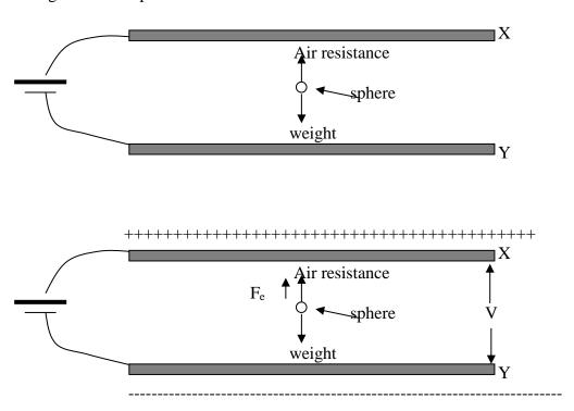
The direction of  $F_e$  depends on the charge on the sphere. Millikan found that the charge on the oil drop was always a multiple of a particular value. I.e. the charge on the oil drop is given by: q = ne, where n is a whole number, and e was  $1.6 \times 10^{-19}C$ . Millikan suggested that 'e' is the charge on an electron. Millikan argued that an oil drop got its charge by gaining or losing electrons, hence the 'e' charge on the drop had to be a whole number times the charge on one electron.
