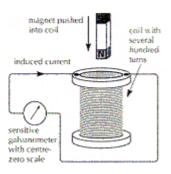
Note: An emf  $(\xi)$  and hence a current, are induced in the solenoid when the magnet is moving into, or out of, the solenoid. The size of the emf  $(\xi)$  depends on the speed of movement and the number of turns on the solenoid, as well as the strength of the magnet.
