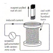
When the magnet is pushed down, the current is clockwise
