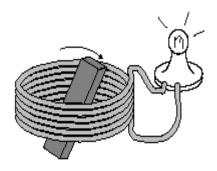
The creation of an electric current in a conductor by changing the magnetic <u>flux</u> is called Electromagnetic Induction. The effect was discovered by the British physicist Michael Faraday and led directly to the development of the rotary electric generator, which converts mechanical motion into electric energy.
