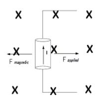
In the diagram, the wire is being moved to the right due to an applied force  $\mathbf{F}_{applied}$ .
