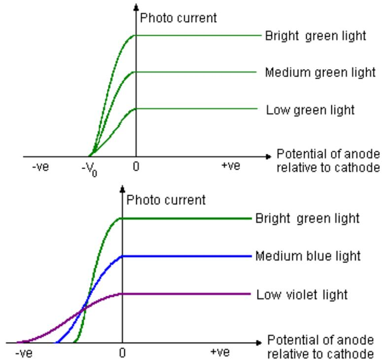
This graph shows that increasing  $V$  does increase  $I$  but the current soon reaches a maximum value called the saturation current.
