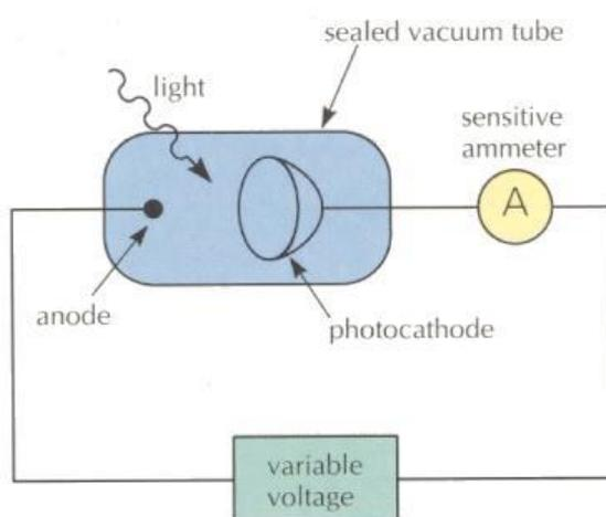
Light radiation falling on the cathode causes emission of electrons, photoelectrons, which are then attracted to the positively charged anode. Thus a current flows. However a current is recorded even when  $V = 0$ .
